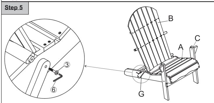
Position Backrest (B) with mortise into housing of Folding Support Bar (G) Secure Folding Support Bar(G) to Backrest(B) using Screw(③) with Allen Wrench(⑥).
