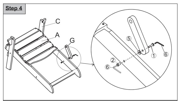
Place the Frame in Step 3 in the position as picture above Attach Folding Support Bar(G) to Seat Panel(A) using Bolt(1), Plastic Washer(5), and Sleeve Nut(2) with Allen Wrench(6).
