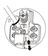
the left. hinge so the hinge pulls closer to the side of the cabinet box, moving the top of the door to needs. If the door seems to be tilting down to the right, turn the side-to-side screw on the top You can adjust one or both hinges on each door, depending on how much correction it
