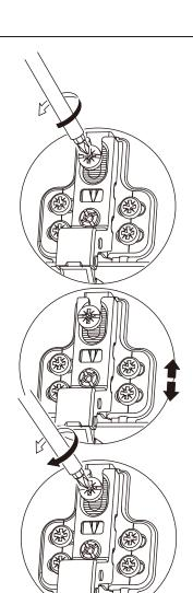
adjust the bottom hinge away from the cabinet. If the door is gapped at the bottom, do the reverse. If the door doesn't meet the box at the top, adjust the top hinge toward the cabinet and/or
