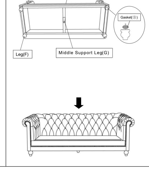
Install the Sofa Leg(F) and the Middle Support Leg(G) onto the bottom of the Sofa by placing one Gasket(③) on the threaded stem.
