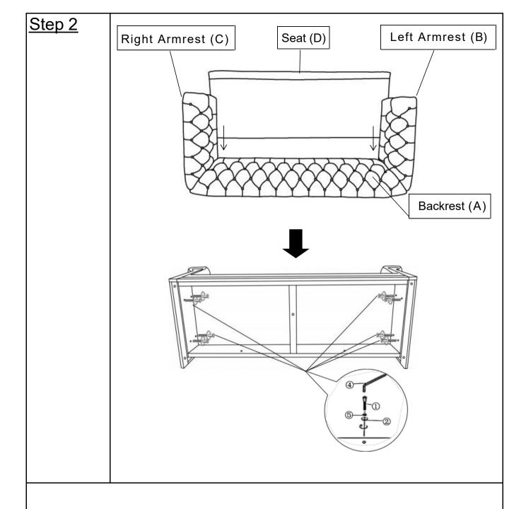
With the assistance from your partner, attach the Seat(D) to the Left Armrest(B) & the Right Armrest(C) using Bolts(①), Spring Washers(⑤), and Washers(②) with the Allen Wrench(④) as pictured above.
