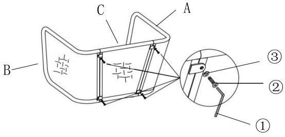
Attach the Left Back Panel (A) and Right Back Panel (B) to the Middle Back Panel (C) using Bolts(2) and Washer (3) with Allen Wrench(1) as the picture shown.
