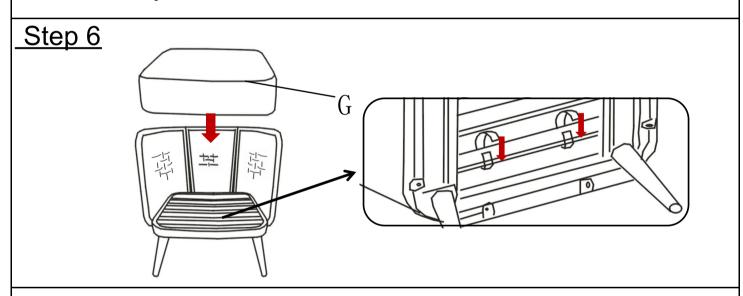
Put the Cushion (G) on to the chair, attach the Magic Tap on the 2 sides to the Seat Panel (D) to fix the Cushion as the picture shown.
