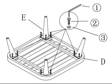
Attach Legs (E) to the Seat Panel (D) using Bolts(②) and Washer (③) with Allen Wrench(①). **DO NOT FULLY TIGHTEN THE BOLTS.**
