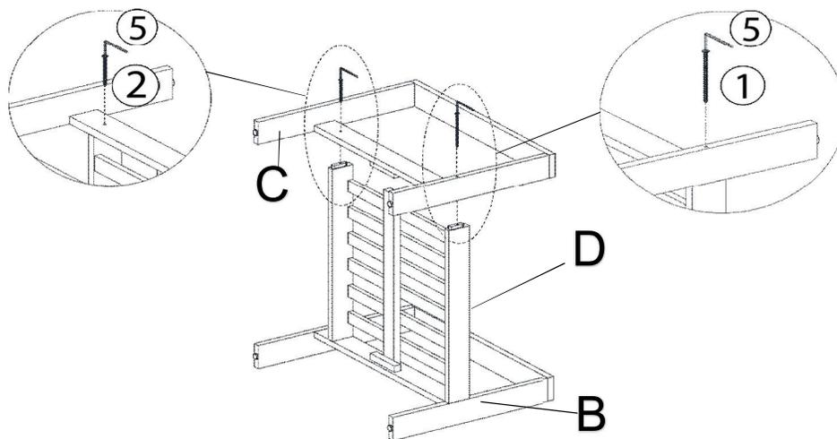
With assistance from your adult partner(s), attach the Left Leg Panel (C) to the assembled parts in Step 2 using Screws (①), Screws (②) and the Allen Wrench (⑤) as pictured
