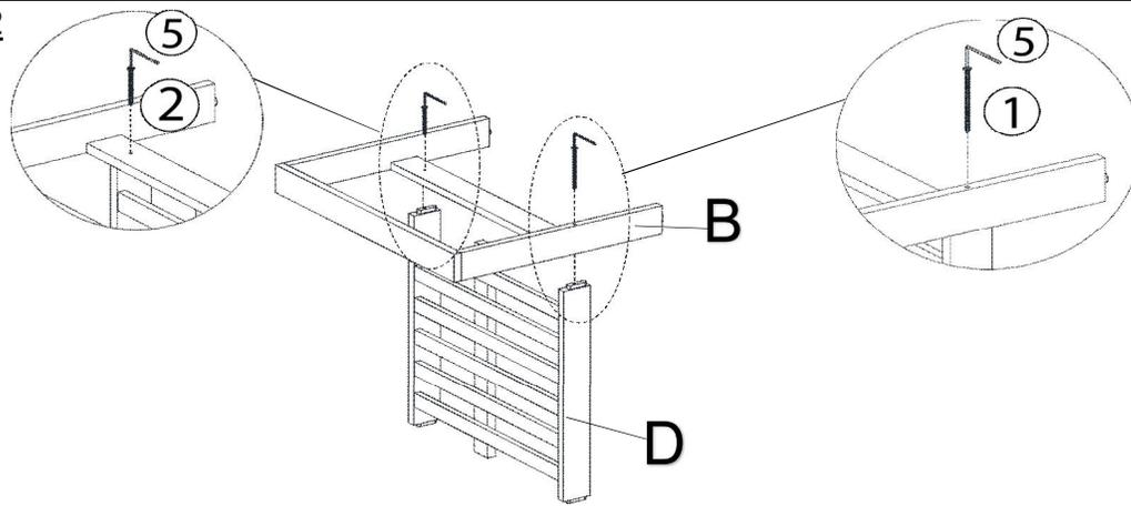
Place the Seat Panel (D) upright as shown in the picture above onto a clean, soft surface to avoid any scratches or damage to the product.
