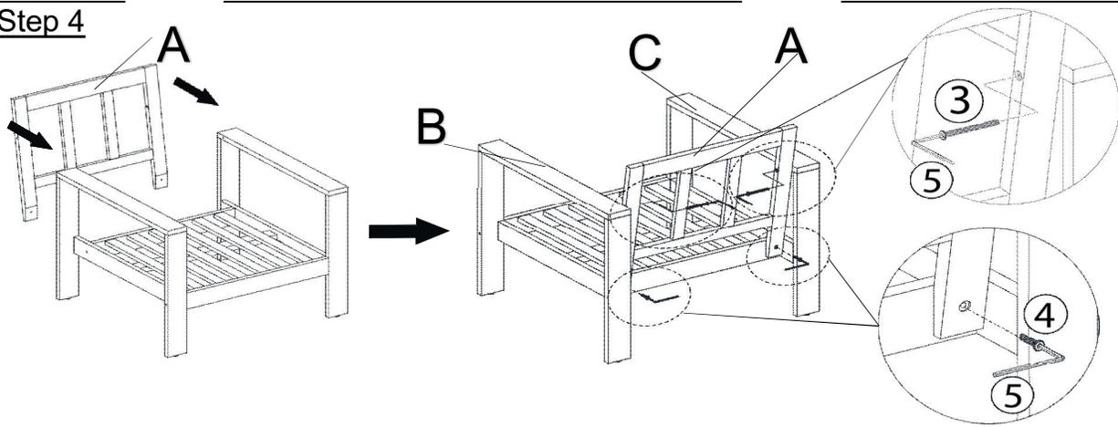
With assistance from your adult partner(s), attach the Backrest Panel (A) to the assembled frame in step 3 by using Bolts (3), Bolts (4) and the Allen Wrench (5) as shown above.
