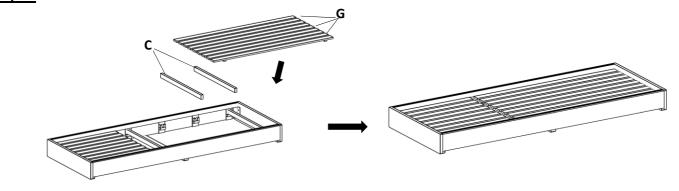
With the help of your adult partner, flip the assembled part in step 6, then attach First Support Bar(C), Seat Frame(G) to assembled part in step 6 as shown above.
