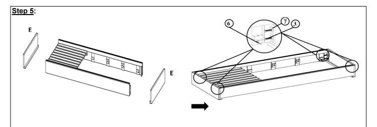
Attach the Seat Base Panel(E) to assembled part in step 4 using Bolt(3), Flat Washer(7) and Allen Wrench(6) as shown above.
