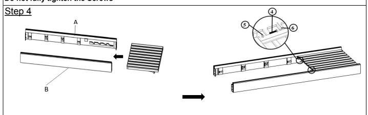
Position the assembled part in step 3 into Left Seat Base Panel(A) and Right Seat Base Panel(B) using Bolt(3), Flat Washer((5)), Allen Wrench((6)) as shown above.
