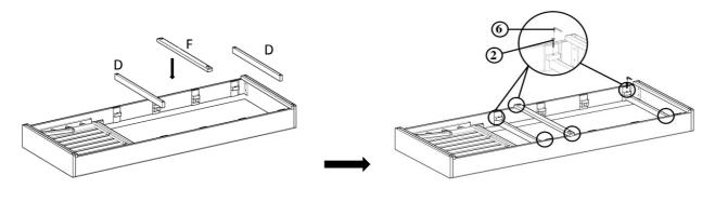
With the help of your adult partner, flip the assembled part in step 5, then attach Second Support Bar(D), Feet Base Panel(F) using Screw(2) and Allen Wrench(6) as shown above. **Do not fully tighten the Screws.**
