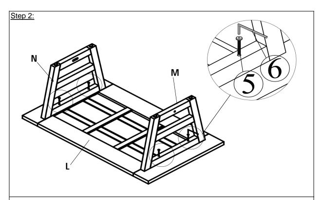
With the help of your adult parter, place the Table Top (L) with its underside skywards onto a clean surface as shown above.
