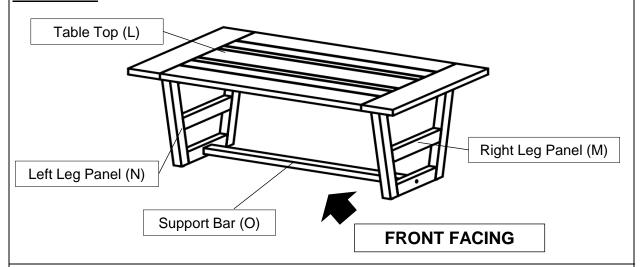
This Table has multiple parts and may require up to 20 minutes to assemble. To give you an overview of the Table parts, the above picture is to help you put the various parts into perspective. Please read through the instructions below to familiarise yourself with the parts and steps before assembly.
