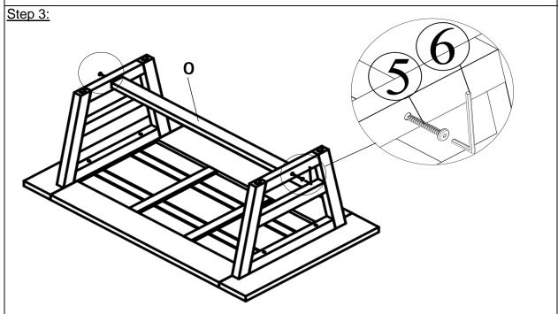
With the help of your adult parter, attach the Support Bar (O) to the assembed part in Step 2 and then secure the Support Bar (O) to the Right Leg Panel (M) and Left Leg Panel (N) by using Screws (⑤) and Allen Wrench (⑥) as shown above.
