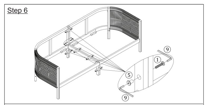
Attach the assembled parts from Step 3 to the assembled parts from Step 5 using the Bolts (1), Sleeve Nut (5) and the Allen Wrench (9). **Do not fully tighten the Bolts.**
