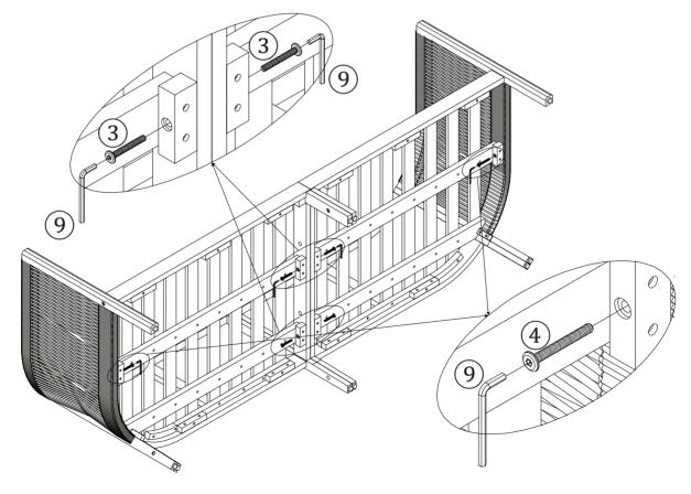
Using the Bolts (3), (4) and the Allen Wrench (9) to secure the assembled parts from Step 6 as shown above.
