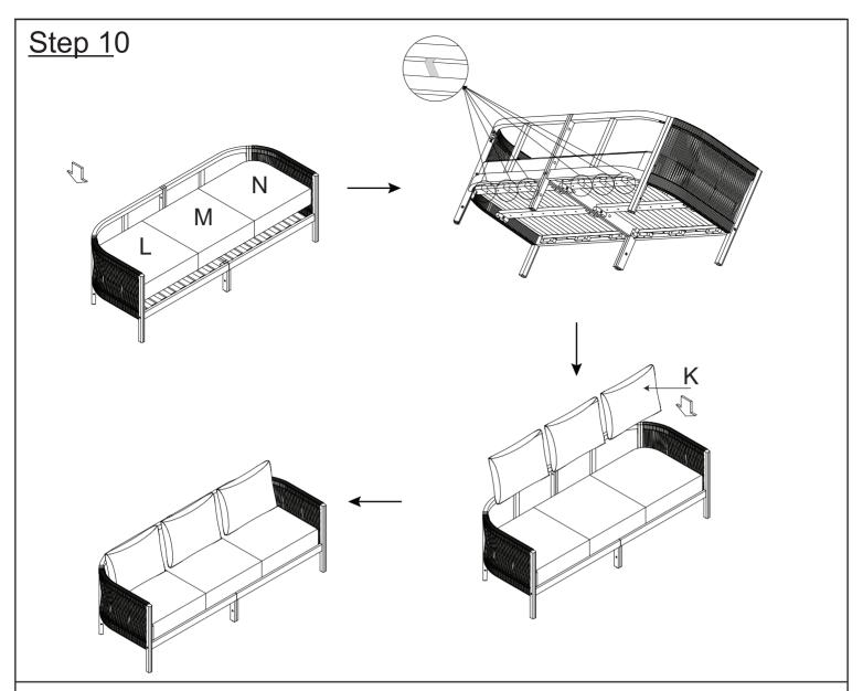
Place the Left Seat Cushion (L), Middle Seat Cushion (M), Right Seat Cushion (N) onto the Bench and affix the magic tape straps around the Bench as shown above.
