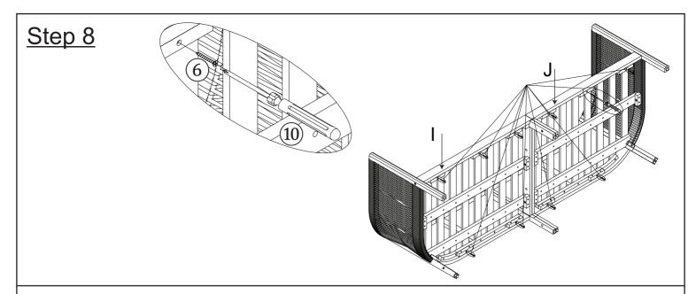
Using the Screws (6) and the Screwdrivers (not provided) (10) to secure the assembled parts from Step 7 as shown above.
