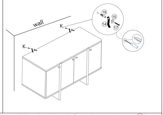
Align the cabinet with the wall and the strip. Screw the expansion screw 18 into the wall and install the flat gasket 15 and screw 17 using the Anti-tipping cloth strip 14 connected to the cabinet. Screw in the tilting strip with a screwdriver 19.
