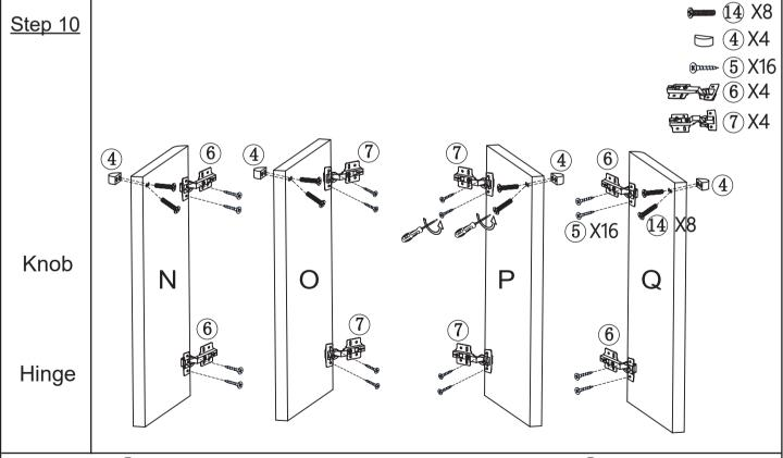
Attach hinge (⑥) to left door panel(N) and right door panel(Q) with screw(⑤) using screwdriver. Attach hinge (⑦) to left door panel(O) and right door panel(P) with screw(⑥) using screwdriver. Attach handle (④) to left door panel(N,O) and right door panel(P,Q) with bolt (⑭) using screwdriver.
