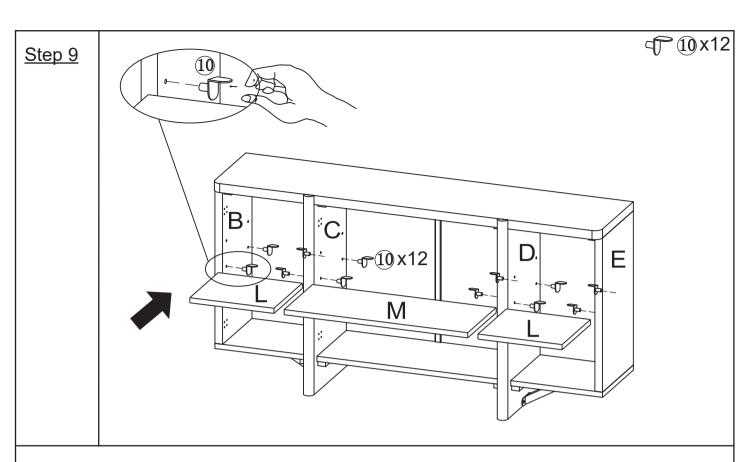
Inset shelf pin(@) into the left side panel(B,C) and the right side panel(D,E).Put left & right adjustable panel(L) and middle adjustable panel(M) on the shelf pin(@).
