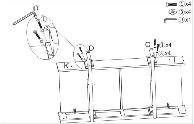
Attach the left bottom panel(I) to the left side panel(C) with bolt(1) and flat washer(3) using allen wrench(1).Attach the right bottom panel(K) to the right side panel(D) with bolt(1) and flat washer(3) using allen wrench(1).
