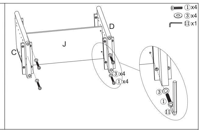
Attach the middle bottom panel(J) to the left side panel(C) with bolt(1) and flat washer(3) using allen wrench(1).
