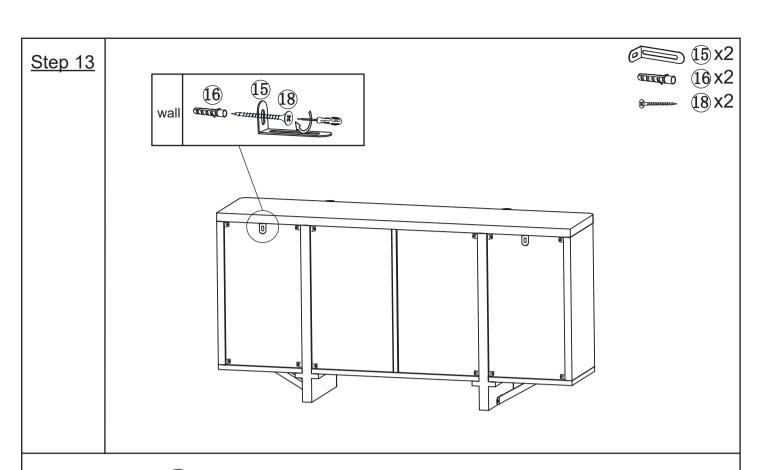
Screw the nut (16) into the wall. Install the short side of anti-tipping iron sheet (15) on the wall with screw(18) using Screwdriver.
