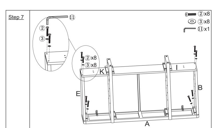
Attach the left side panel(B) to the top panel(A) and the left bottom panel(I) with bolt(2) and flat washer(3) using allen wrench(1). Repeat the previous steps to the right side panel(E).
