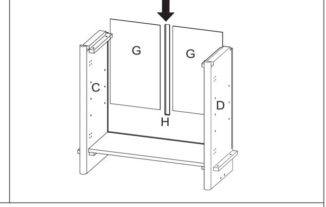
Insert the back panel(G) into the groove of the left side panel(C) and the right side panel(D).
