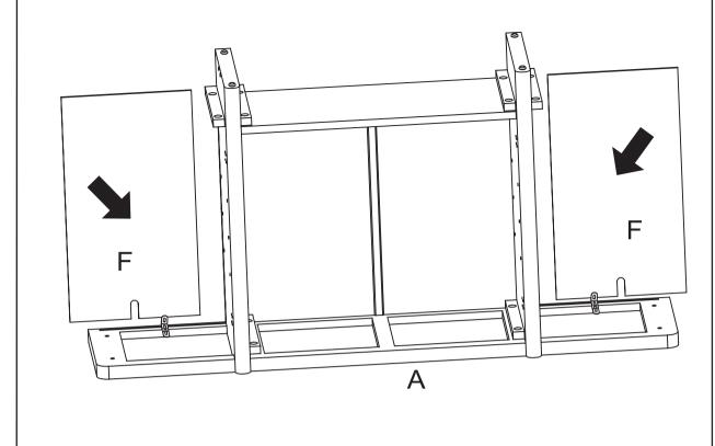
Insert the back panel(F) into the groove of the top panel(A).
