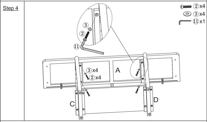
Attach the top panel(A) to the left side panel(C) with bolt(2) and flat washer(3) using allen wrench(1).
