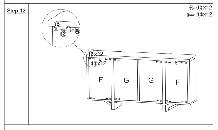
Attach plastic button(12) into the back panel(F,G) with Screw(13) using Screwdriver.
