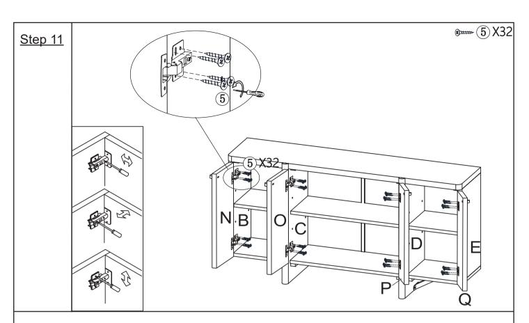
Attach left door panel(N,O) to left side panel (B,C) with screw(5) using screwdriver.Repeat the previous steps to right door panel(P,Q).
