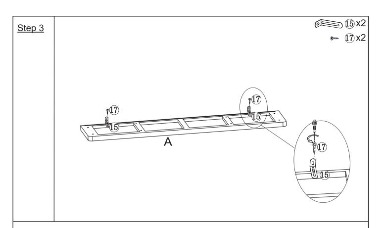
Attach the long side of anti-tipping iron sheet ((15)) into the top panel (A) with screw ((17)) using screwdriver.
