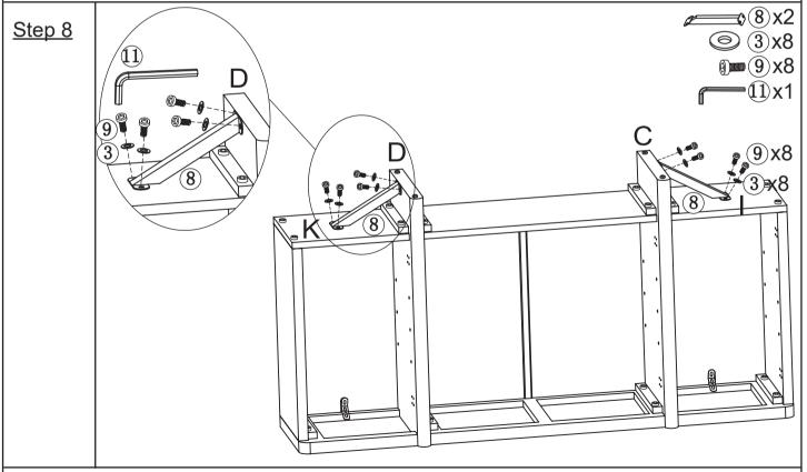
Attach the metal support strip(\$) to the left side panel(C) and the left bottom panel(I) with bolt(\$) and flat washer(\$) using allen wrench(\$). Repeat the previous steps to the right side panel(D) and the right bottom panel(K).
