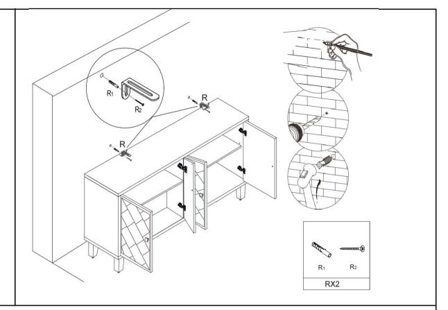
Align the cabinet with the wall and slats. Screw the expansion screw (R1) into the wall, then attach the other end of the Sheet Iron (Q) to the expansion screw (R1) on the wall and tighten the screw (R2) to ensure that the anti-tipover device is securely mounted and effective in preventing the cabinet from tipping over.
