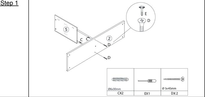
1. Take the Middle panel 5 and the Bottom panel 2, align the bottom panel with the bottom edge of the Middle panel, insert the Wood dowel (C) into the corresponding hole in the connection are a between the middle panel 5 and the bottom panel 2, and use a screwdriver (E) to tighten the screws (D) to make sure that the connection is secure.
