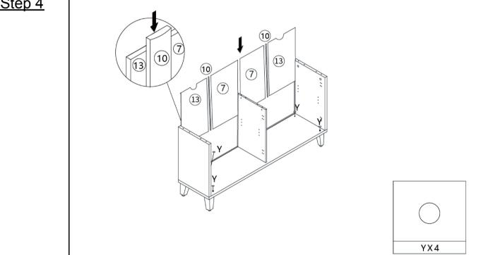
Insert the back panels 7 13 and connect them with the back panel strip 10 in the center.
