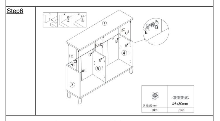
Connect top panel(①) and two side panels(③④)&middle side panel(⑤), with Wood dowel (C), Cam lock nut(B). Next, use a screwdriver(E) to rotate the Cam lock nut(B).
