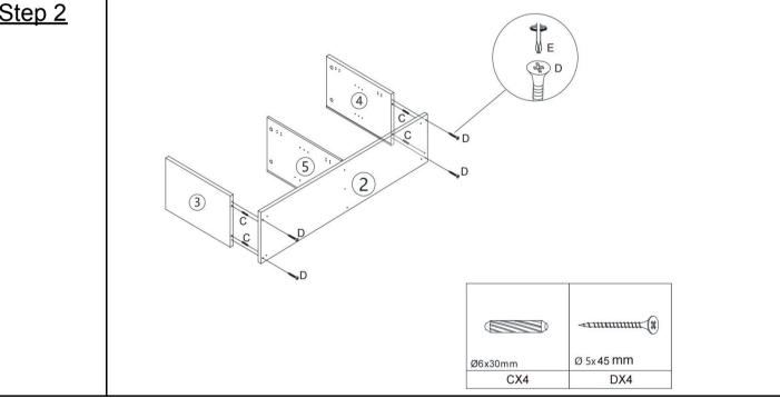
1. Take the left side panel ③ and the right side panel ④, align the bottom panel with the bottom edge of the side panels, insert the Wood dowel (C) into the corresponding hole in the connection area between the side panels ③ ④ and the bottom panel ②, and use a screwdriver (E) to tighten the screws (D) to make sure that the connection is secure.
