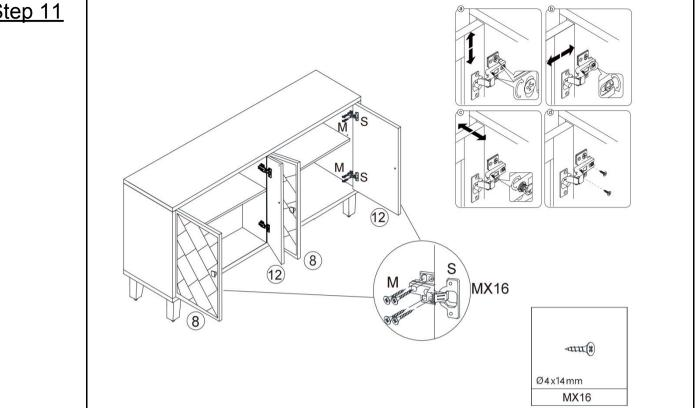
Install the left door  $\circledR$  on the Left Side Panel, Install the right door ข on the Right Side Panel.
