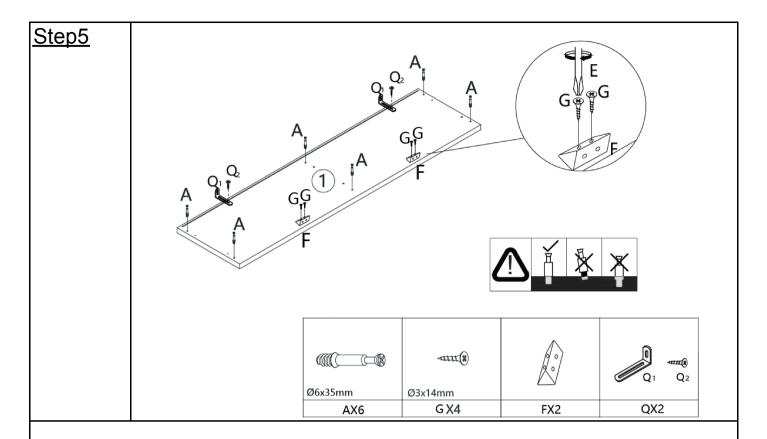
Mount cam lock bolt (A), Door Stopper (F), and Sheet Iron (Q) on top panel. (1)
