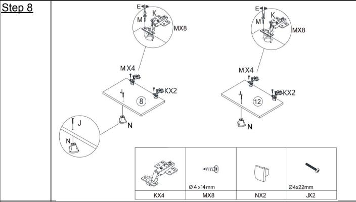
Installation of hinges (K) and Pull handle (N) on Doors (8),(12) .
