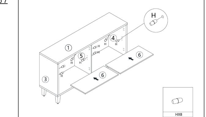
Insert shelf nails(H) on two side panels(34)and the middle panel(5), then place layer panels(6).
