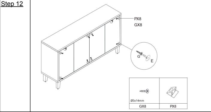
Fit back panel bracket (P) on the back of the cabinet with screws (G).
