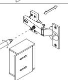
If the door gap is large, you can adjust the hinges left and right
