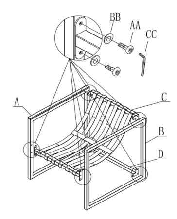
**Step 1:** Assemble armrest parts A and B to seat parts C and D with screws. Please do not lock the screws when assembling. Lock all screws when you complete step 1.
