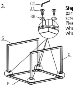
**Step 3:** Assemble the table foot part G to the table frame F with screws.
