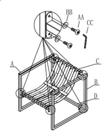
**Step 1:** Assemble armrest parts A and B to seat parts C and D with screws. Please do not lock the screws when assembling. Lock all screws when you complete step 1.
