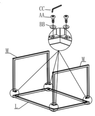
**Step 5:** Fasten the table foot part M to the table frame L with screws.
