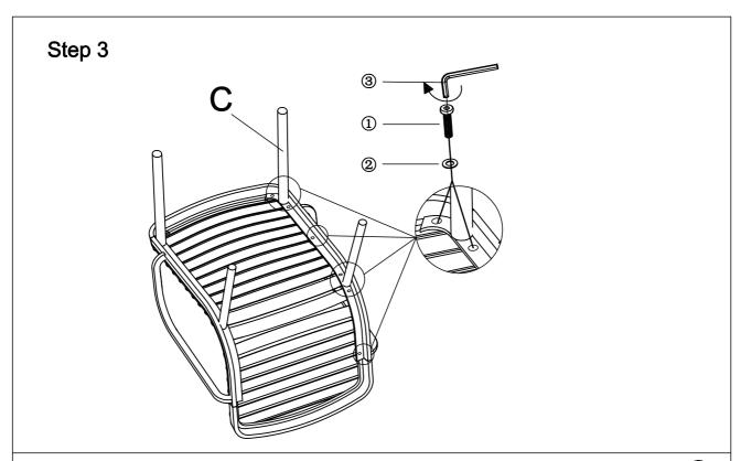
Attach the Right Leg (C) to the Chair Seat and Back (A), using Bolts(1) and Washer(2) with Allen Wrench(3).
