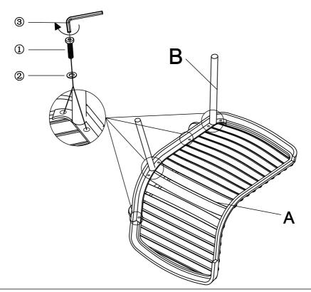
Attach the Left leg (B) to the Chair Seat and Back (A), using Bolts(1) and Washer (2) with Allen Wrench (3) as shown above.
