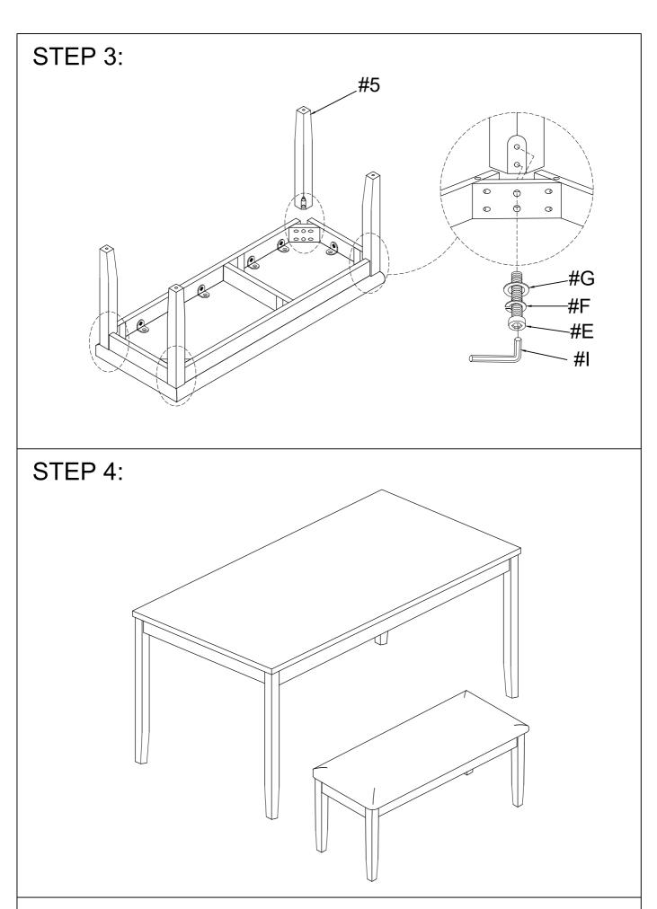
Tighten all screws until completely asembled.
