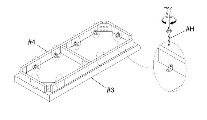
Do not tighten screws until completely asembled.
