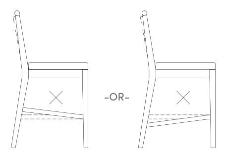
Re-check to confirm that the proper legs are installed in their intended position on the proper side of the stool.
