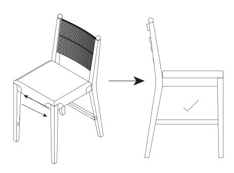
Carefully flip the stool over on a flat surface and make sure the legs are touching the ground evenly before tightening everything to 100%.
