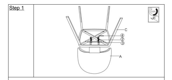
Attach the Chair Frame (C) to Chair Back(A) using the washer(③), Bolt(②) with Allen Wrench(④) as pictured above. Do not fully tighten the Bolts.
