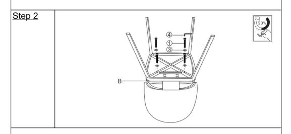
Attach the Seat Cushion (B) to Chair Frame (C) using the washer (3), Bolt(1) with Allen Wrench(4) as pictured above. Do not fully tighten the Bolts.
