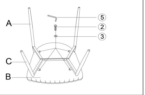
Turn the cushion (B) over, bottom side up, then invert the assembly from the previous step (A) (C) onto the cushion (B).( shown in the figure).Insert screw ② through washer ③ and attach the rack to the seat cushion (B) through the holes in the rack (as in the figure). If the screw turns with resistance, tap the frame to align the hole with the screw, then tighten it.
