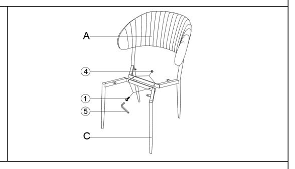
Place the backrest(A) and the front legs (C) as shown in the figure, align the middle two holes.
