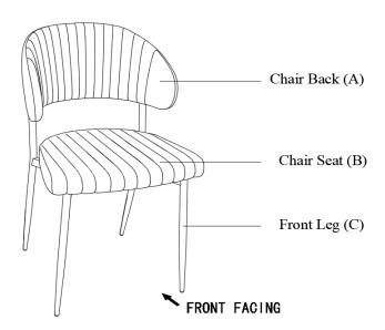
This Chair has multiple parts and may require up to some 30 minutes to assemble. To give you an overview of the Chair parts, the above picture is to help you put the various parts into perspective. Please read through the instructions below to familiarise yourself with the parts and steps before assembly.
