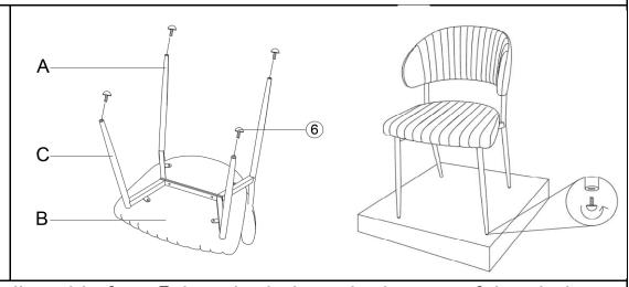
Screw the adjustable foot ⑥ into the hole at the bottom of the chair leg.(As shown in the figure)
