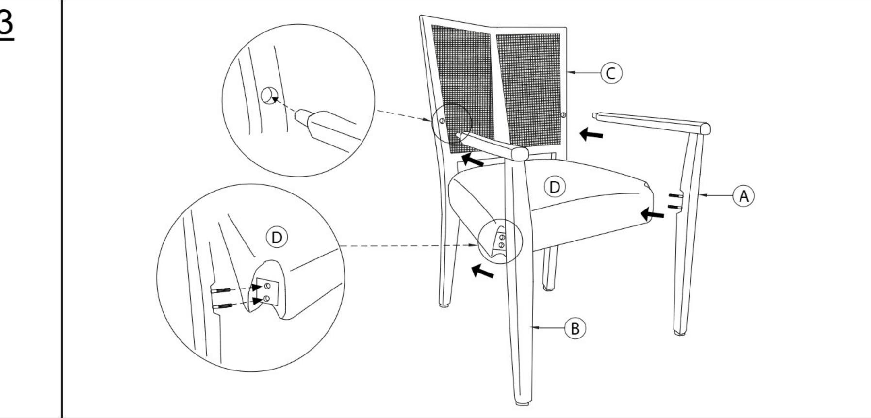
Attach the both Arm leg (A) and (B) into the Seat Cushion (D) and Chair back (C) as pictured above.
