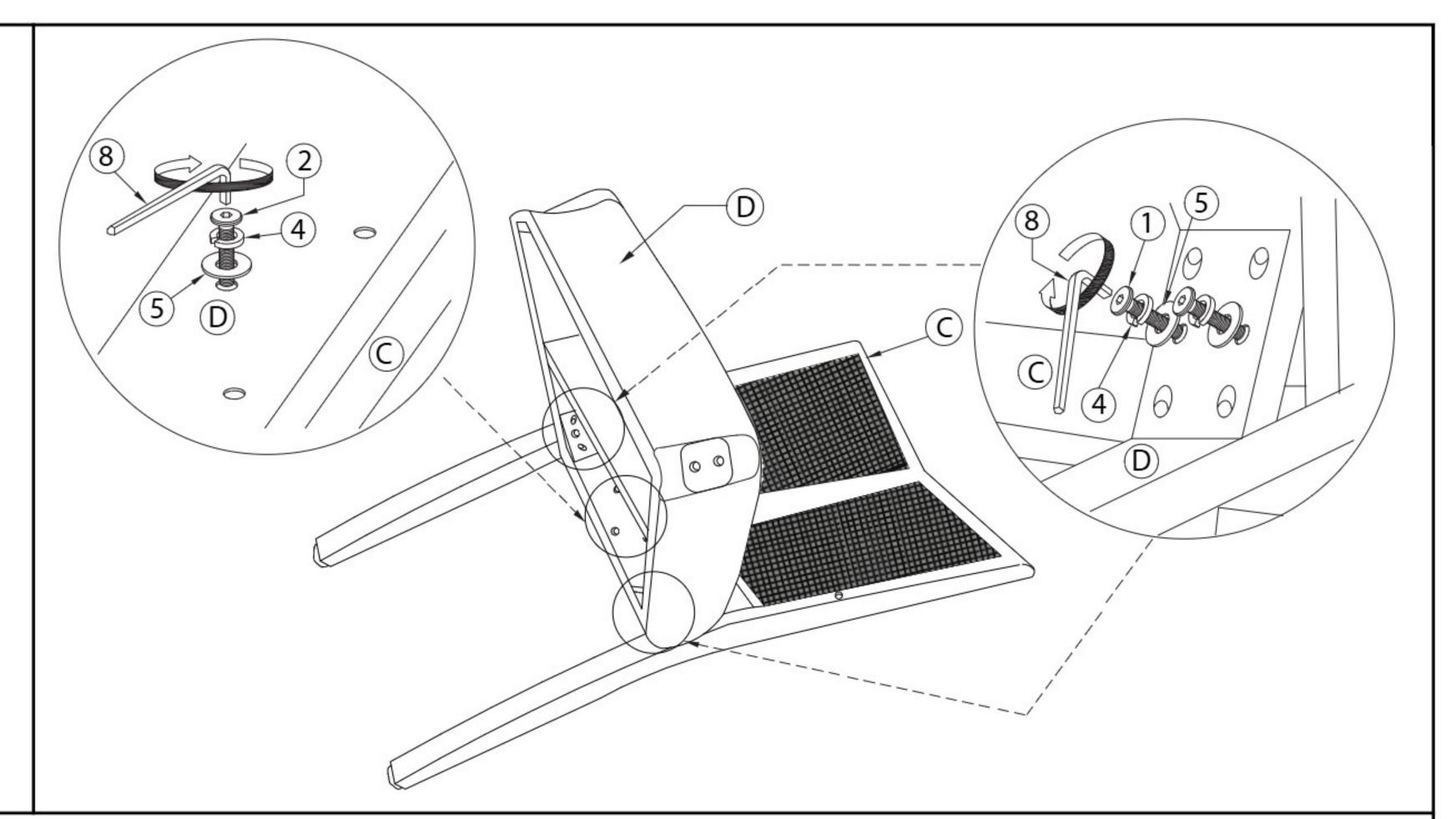
Place the Chair back (C) on a clean , non-marking surface. Install the Seat Cushion (D) into the Chair back (C) using JCBC Screw (M6\*80mm) ①, and JCBC Screw (M6\*35mm) ②, Spring washer (M6) ④, Flat washer (M6) ⑤, with Allen Key (M4) ⑧, as pictured above.
