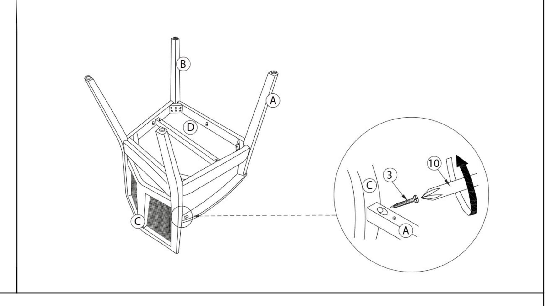
Install both Right arm leg (A) and Left arm leg (B) with the Chair back (C) using CSK Screw (M4\*45mm) ③, with Screw driver ①, as pictured above.
