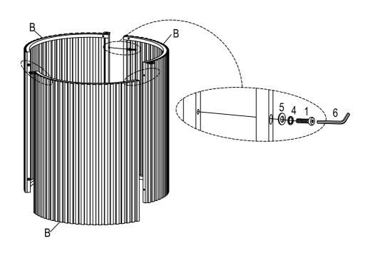
Note: At this stage, do not fully tighten the bolts .
