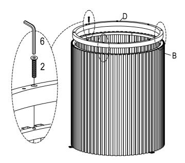
Note: At this stage, do not fully tighten the bolts .
