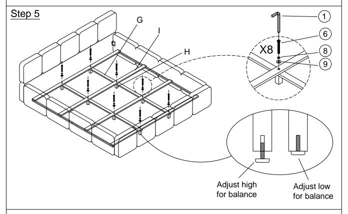
Attached Middle support leg (H) and Center support bar (G) to Slats (I) by using Bolt (6), Spring Washer (8), Flat Washer (9) and Allen Wrench (1).
