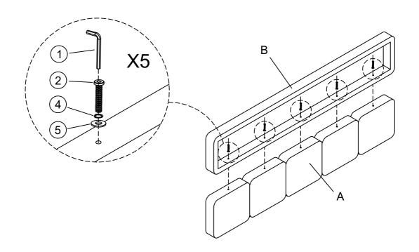
Attached Bottom board (A) to Head board (B) by using Bolt (2), Spring Washer (4), Flat Washer (5) and Allen Wrench (1).
