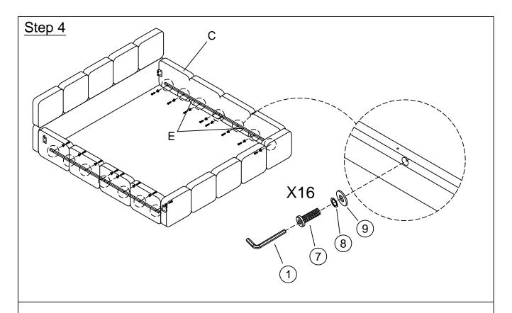
Attached Side support bar (E) to Side rail (C) by using Bolt (7), Spring Washer (8), Flat Washer (9) and Allen Wrench (1).
