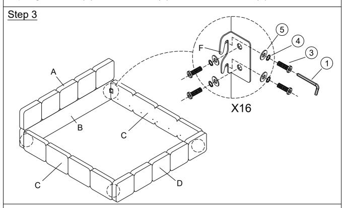
Attached Side rail (C) and Foot board (D) to Bottom board (B) by using Bolt (3), Spring Washer (4), Flat Washer (5), Connector (F) and Allen Wrench (1).
