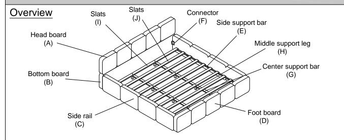
This Upholstered Bed has multiple parts and may require up to some 30 minutes to assemble. To give you an overview of the Upholstered Bed parts, the above picture is to help you put the various parts into perspective. Please read through the instructions below to familiarise yourself with the parts and steps before assembly.
