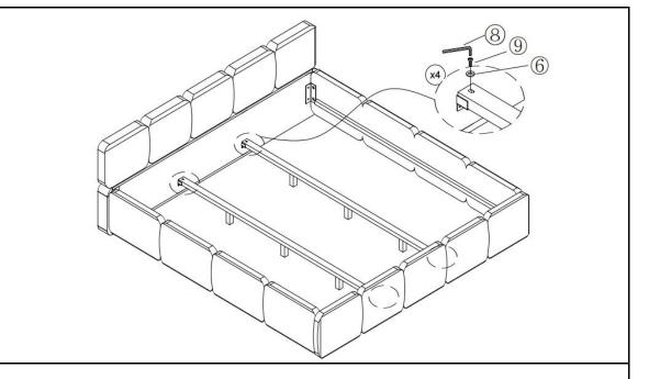
Attached Center support bars (E) to Center support bar fittings (H) by using Bolt ( (9) ) 、 Flat Washer ( (6) ) and Allen Wrench ( (8) )
