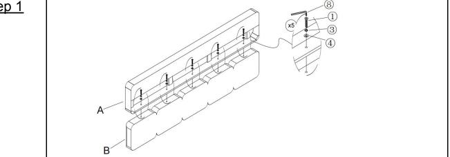
Attached Bottom board (A) to Head board (B) by using Bolt (1), Spring Washer (3) Tlat Washer (4) and Allen Wrench (8)
