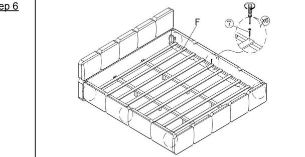
Attached Slats (F) to Side rail (C) by using Screw (⑦)
