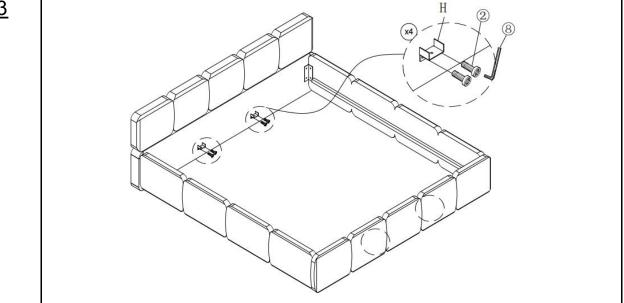
Attached Center support bar fittings ( H ) to Foot board ( D ) and Bottom board ( A ) by using Bolt ( ② ) and Allen Wrench ( ⑧ )
