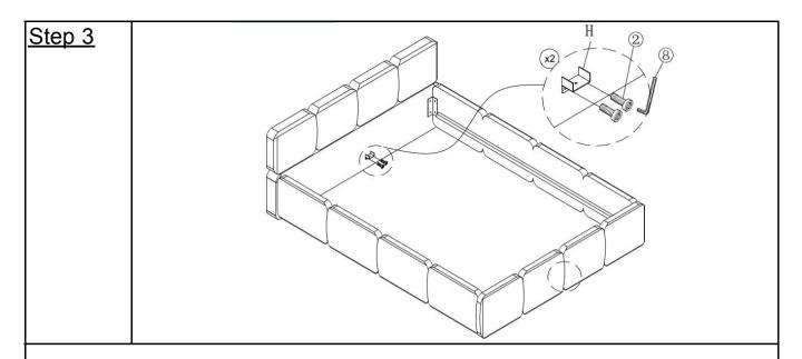
Attached Center support bar fittings ( H ) to Foot board ( D ) and Bottom board ( A ) by using Bolt ( ② ) and Allen Wrench ( ⑧ )
