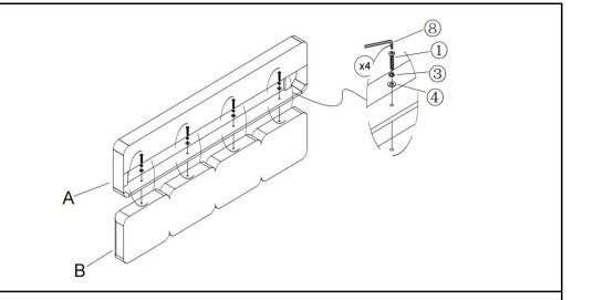
Attached Bottom board (A) to Head board (B) by using Bolt (1), Spring Washer (3), Flat Washer (4) and Allen Wrench (8)
