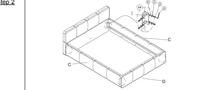
Attached Side rail (C) and Foot board (D) to Bottom board (A) by using Bolt (②)、Spring Washer (⑤)、Flat Washer (⑥)、Connector (I) and Allen Wrench (®)
