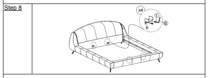
Attach Center support bar fittings(K) to Headboard(A) and Footboard(D) by using Bolt (1) and Allen Wrench (6), as pictured above.
