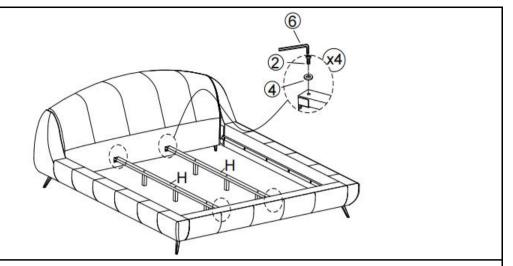
Attach Center support bar(H) to Iron Center support bar fittings(K) by using Bolt (②), Flat Washer(④) and Allen Wrench (⑥), as pictured above.
