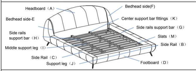
This Upholstered Bed has multiple parts and may require up to some 30 minutes to assemble. To give you an overview of the Upholstered Bed parts, the above picture is to help you put the various parts into perspective. Please read through the instructions below to familiarise yourself with the parts and steps before assembly.
