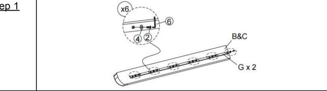
Attached Side rails support bar (G) to Side Rail(B&C) by using Bolt (2) Flat Washer (4) and Allen Wrench (6), as pictured above.
