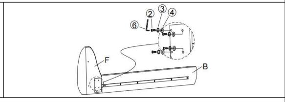
Attach Bedhead side(F) to Side Rail(B) by using Bolt (2), Spring Washer (3), Flat Washer (4) and Allen Wrench (6), as pictured above.
