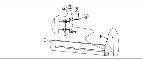
Attach Bedhead side(E) to Side Rail(C) by using Bolt (②), Spring Washer (③), Flat Washer (④) and Allen Wrench (⑥), as pictured above.
