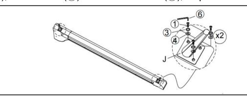
Attach Support leg(J) to Side Rail(C) by using Bolt (1), Spring Washer (3), Flat Washer (4) and Allen Wrench (6), as pictured above.
