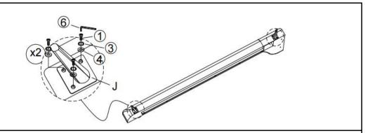
Attach Support leg(J) to Side Rail(B) by using Bolt (1), Spring Washer (3), Flat Washer (4) and Allen Wrench (6), as pictured above.
