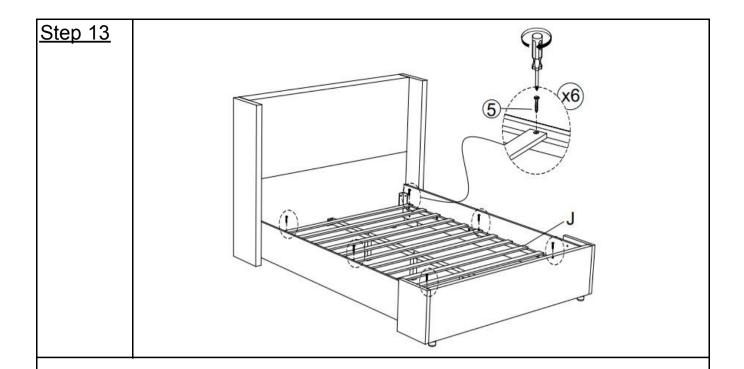
Attach Bed Slat(J) to Side tray(I) by using Screw(⑤), as pictured above.
