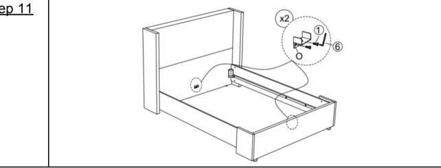
Attach Iron Bracket(O) to Headboard B(B) and Bed End(G) by using Bolt (1) and Allen Wrench (6), as pictured above.
