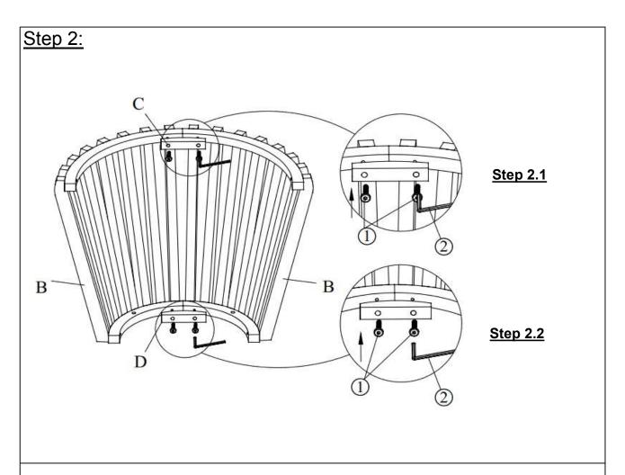
Attach two Leg Panels (B) together and then:
