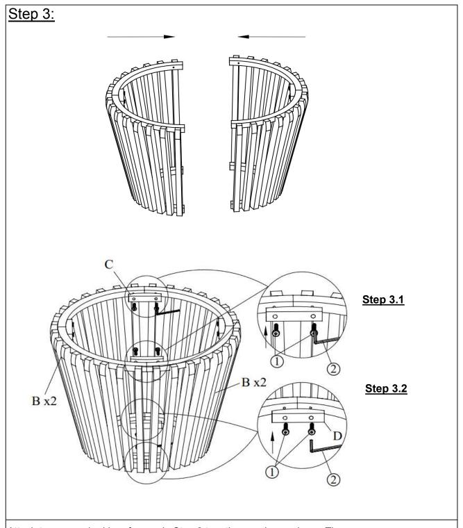
Attach two assembed Leg frames in Step 2 together as shown above. Then:
