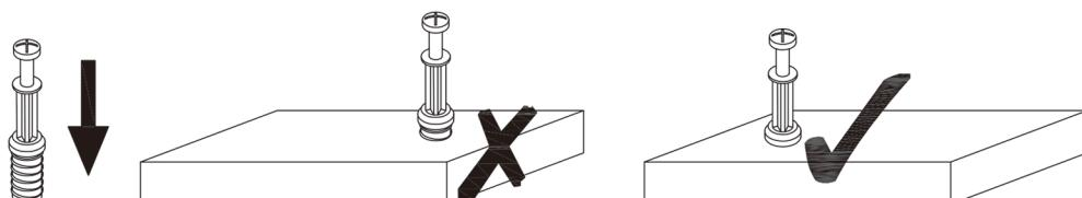
Tighten quickfit until shoulder is flush with panel. Do not overtighten or undertighten.
