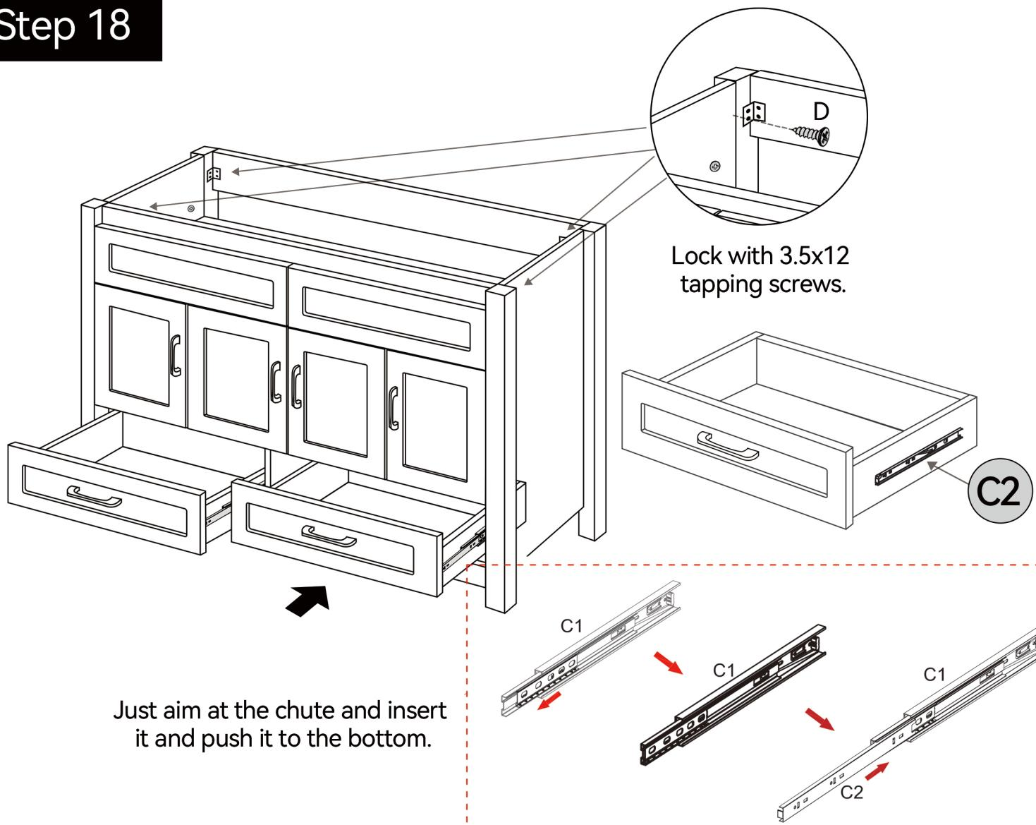
Just aim at the chute and insert it and push it to the bottom.
