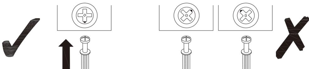
When fitting cam lock, ensure starting position is correct before you insert connecting quickfit.
