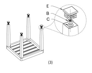
**Step 4**: Do not over tighten bolts, it will cause the damage of product without warranty; Your table should be ready for use. If your table is not stable, double check your assembly procedure or loosen some bolts and tighten them again.
