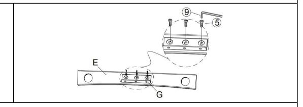
Attached Iron sheet (G) to Back Stretcher (E) by using Bolt (⑤) and Allen wrench (⑨), as pictured above.
