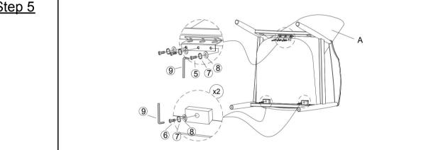
Attached Seat Frame (A) to Front Stretcher (D) by using Bolt (6), Spring Washer (⑦), Flat Washer (⑧), Allen Wrench (⑨) and to Back Stretcher (E) by using Bolt (⑤), Spring Washer (⑦), Flat Washer (⑧) and Allen Wrench (9), as pictured above.
