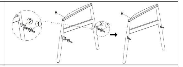
Install the Full Thread Screw (1) and Wood Dowel (2) on the Right Arm (B), as pictured above.
