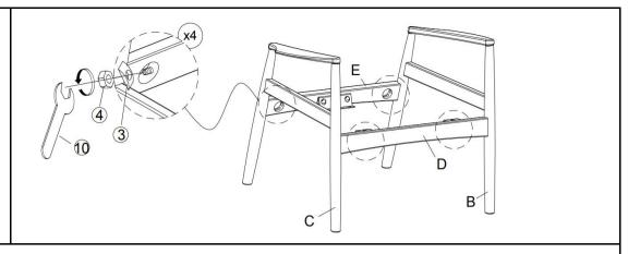
Attached Front Stretcher (D) and Back Stretcher (E) to Left Arm (B) and Right Arm(C) by using Half Moon Washer (3), Nut (4) and Open wrench (10), as pictured above.
