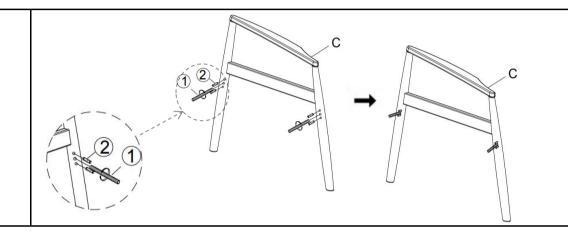
Install the Full Thread Screw (1) and Wood Dowel (2) on the Left Arm (C), as pictured above.
