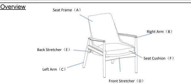
This chair has multiple parts and may require up to some 30 minutes to assemble. To give you an overview of the chair parts, the above picture is to help you put the various parts into perspective. Please read through the instructions below to familiarise yourself with the parts and steps before assembly.
