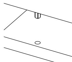
When joining two panels together, don't forget to gently hit the panels to adjust the joint.
