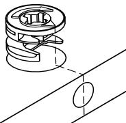
You should insert these cams with the little arrow pointing towards the drilling on the panel's edge (shown on the left).
