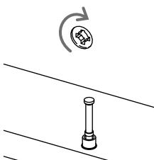
This is a spreading bolt. You should put it with the black plastic part facing down.
