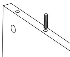
Put in the dowel inside the indicated hole and softly hit it until it's fully inside.
