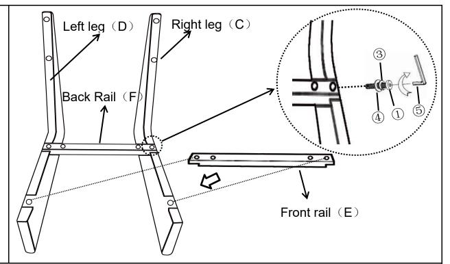
Attach the Rails(E+F) into the mounting positions of the Legs(C+D) using Bolts(1),Spring Washer(3) and Washer(4) with Allen Wrench(5). Fully tighten the Bolts.
