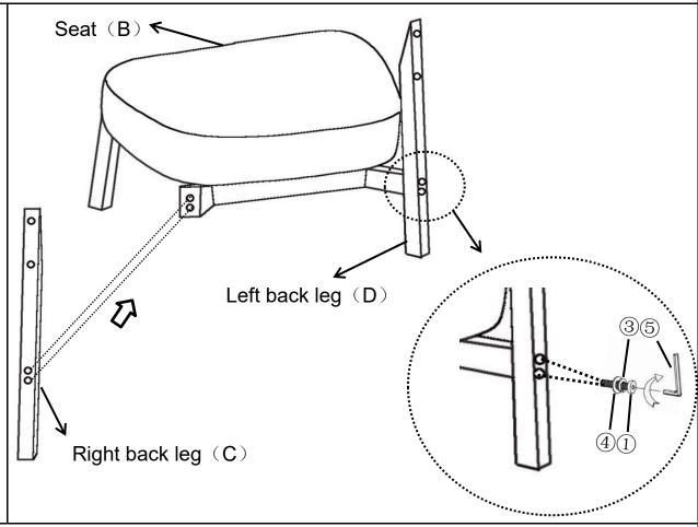
Attach the two Back Legs(C+D) into the mounting positions of the Seat(B) using Bolts (①), Spring Washer(③) and Washer(④) with Allen Wrench (⑤). Do not fully tighten the Bolts.
