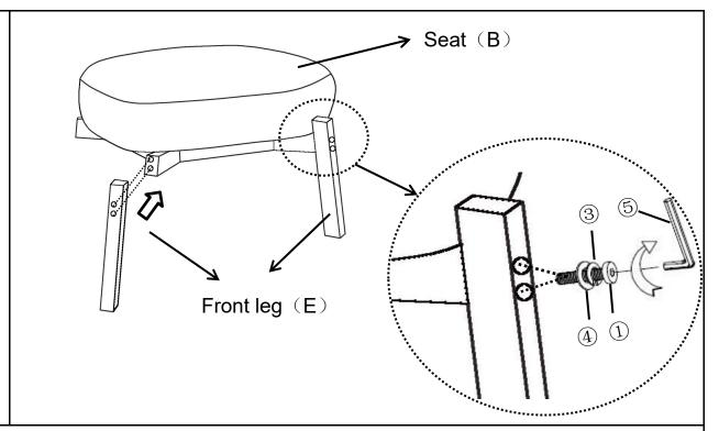
Put the Seat(B) and Front legs (E) onto a clean, non-marring surface. Attach the two Front Legs(E) into the mounting positions of the Seat(B) using Bolts(1), Spring Washer(3) and Washer(4) with Allen Wrench (5).
