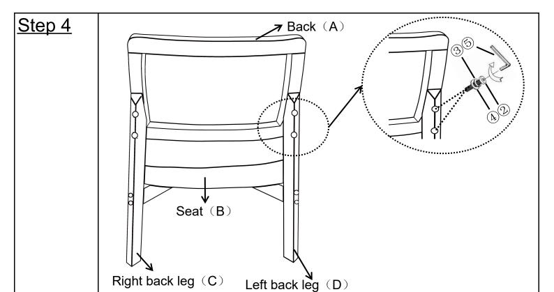
Attach the Back Legs(C+D) into the mounting positions of the Back(A) using Bolts(②), Spring Washer(③) and Washer(④) with Allen Key(⑤).
