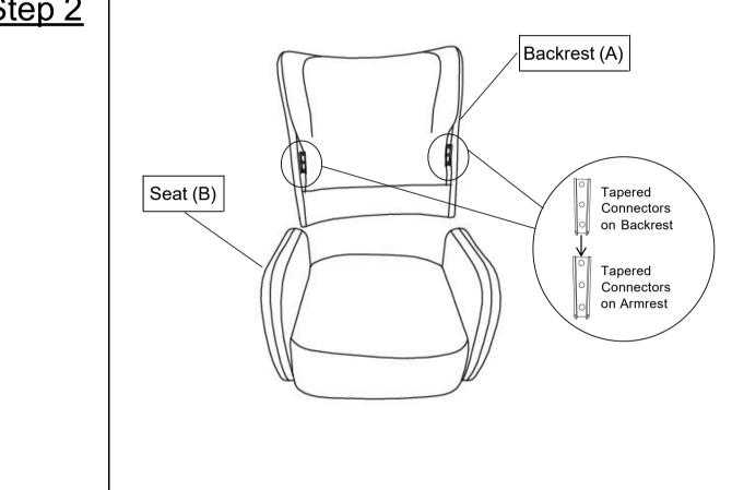
With assistance from an adult partner, lift the Backrest(A) up. Align the Tapered Connectors on the Backrest(A) and the Seat(B).
