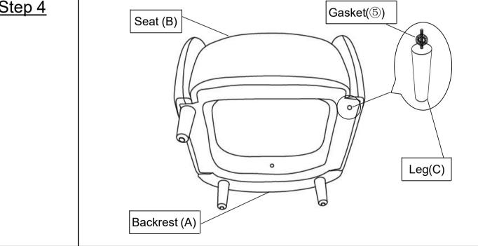
Install the Leg(C) onto the bottom of the Chair by placing one Gasket(⑤) on the threaded stem. Then insert the threaded stem into the threaded mounting postion at the corner of the Chair. Tighten by turning the Leg clockwise.
