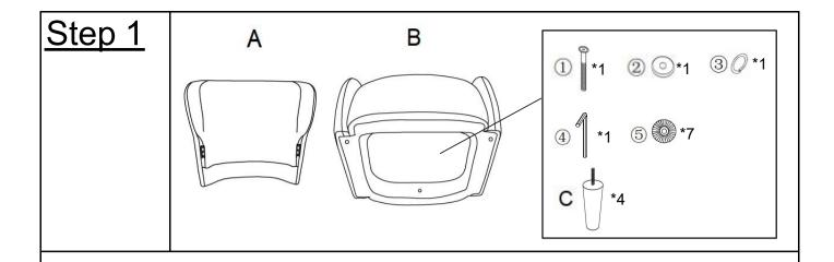
Position the Backrest(A) and Seat(B) on a clean, non-marring surface, as shown. Do not place on surface that can scratch or damage the upholstery.
