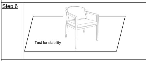
Position the Chair on a level surface and test for stability. If the Chair is not Stable, fully tighten the Bolits.
