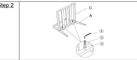
Place the Right Armrest(A) and Seat Board(C) on a clean ,non-marring surface. Attach Right Armrest(A) to Seat Board(C) using Bolts(2), and Washer(3) with Allen Wrench(4).
