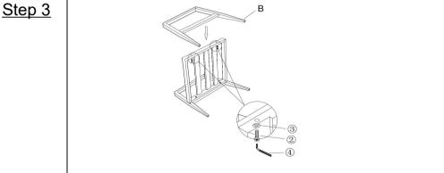
Attach Left Armrest(B) to Seat Board(C) using Bolts(2),and Washer(3) with Allen Wrench(4).
