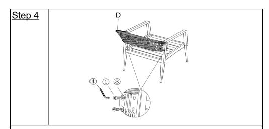
Attach Backrest (D) to Right Armrest (A) and Left Armrest(B) and Seat Board(C) using Bolts(1),and Washer(3) with Allen Wrench(4).
