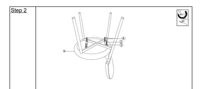
Attach the Seat Cushion (B) to Leg Frame (C) using the Washer (③), Bolt (②) with Allen Wrench (④) as pictured above.
