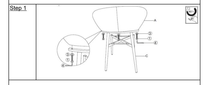
Attach the Back (A) to Leg Frame (C) using the Washer (③), Bolt (①) with Allen Wrench (④) as pictured above.
