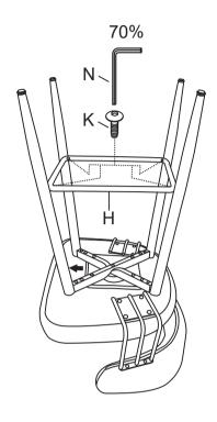
STEP 11 In this step please tighten all bolts (L,M,K) 100% by alley key (N) as shown in below diagram.
