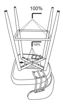
**STEP 12** Please recheck and ensure 100% tighten all the bolts in this step. After initial assembly, the product may acclimate to its new environment. Please ensure all bolts are still securely tightened.
