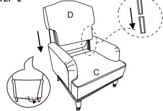
Carefully align male and female metal bracket then push all the way down to secure. Smooth the lower back flap and carefully secure the velcro belt to rear bottom edge of seat frame.
