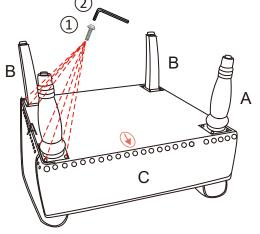
Attach the front and rear feet to the bottom of the seat frame.
