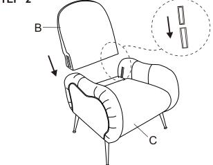
Install the chair back onto the seat frame.
