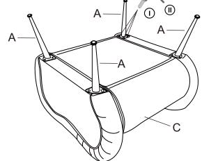
Install the chair legs at the bottom of the seat frame.
