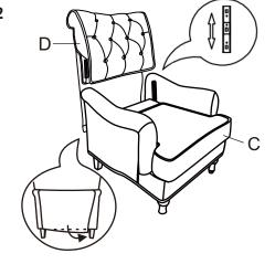
Carefully align male and female metal bracket then push all the way down to secure. Smooth the lower back flap and carefully secure the velcro belt to rear bottom edge of seat frame.
