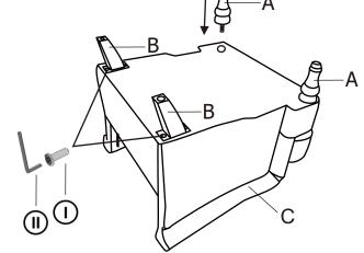
Attach the front and rear feet to the bottom of the seat frame.
