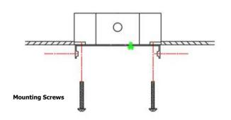
STEP 3 Put the mounting unit into the junction box, fixed it with the mounting screws.
