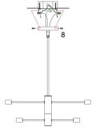
STEP 5 Install the fixture to the junction with the screws.
