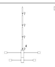
Step 2: Put the wire into the tube L300&L500 tube, and put the lamp body into the canopy as right top instruction.
