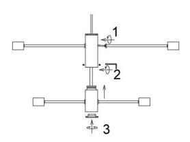
Step 1: Loosing the nuts(2) by the spanner, put the tube(1) into the lamp body, if the wire is too long, please adjust the wire by opening the bottom cap as above instruction.
