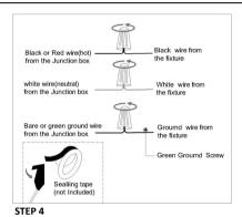
Make the electrical connection from the junction box to the fixture Connect the ground wire to the mounting unit using the preinstalled green ground srews
