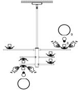
Step 6 Install the light bulb, then put the glass into the socket as
