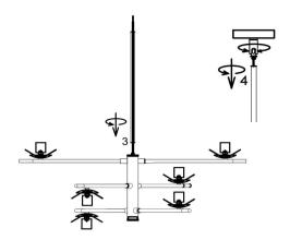
Step2: Put the wire into the L600 tube, then put the tube into the fixture.Meanwhile, install the L600 tube into the canopy.
