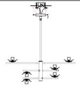
Step 5 Install the fixture to the junction with the screws.
