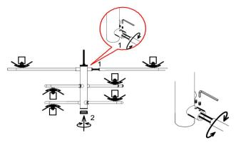
Step1:Open the nuts by the wrench, then put the tube into the fixture and locked it with the nust. If the wire is too long then making it hard to put in the tube, you can open the bottom cap, to fix the wire then install the tube again.
