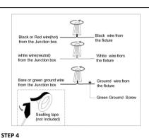
Make the electrical connection from the junction box to the fixture. Connect the ground wire to the mounting unit using the preinstalled green ground screws.
