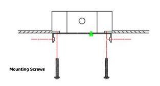
Step 3 Put the mounting unit into the junction box, fixed it with the mounting screws.
