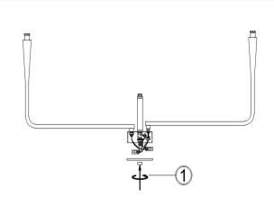
**STEP 1.** Adjust the distance between the lamp arms to be even, connect the internal line of the lamp body, do a good job of insulation, and lock the nut of the lamp arm in the lamp gu, and lock the lamp cover
