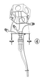
**STEP 4** Fix the hanging plate on the ceiling embedded part with screw 1, and ensure that the installation is firm
