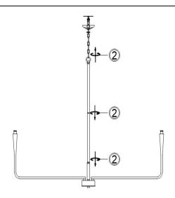
**STEP 2.** After the main line of the lamp body passes through the tube, the tube is twisted on the lamp body, and the lamp body part is fully assembled.
