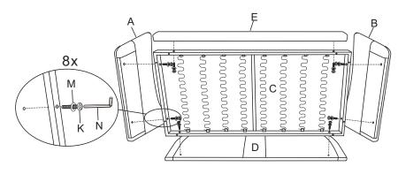
1. Connect sofa arms(Part A&B), Back Frame(Part D), Seat Frame(Part C), Wood Piece(Part E), then install the screws(Part K) & gaskets (Part M) with Toll ( Part N ).
