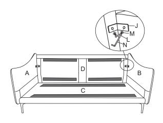
3.Connect the back frame (Part D) by aligning the metal piece (Part J) on Arms (Part A&B), then install Screw (Part L) & gaskets (Part M) with Toll (Part N)
