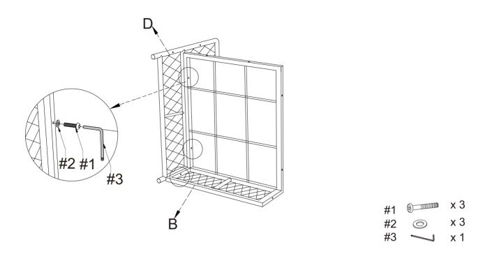
Step 2. Attach left arm panel (part C) to seat panel (part B) using bolts (part #1), flat washers (part #2) and allen wrench (part #3).
