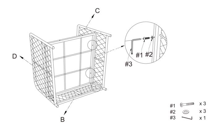
Step 3. Attach back panel (part A) to assembled unit (parts B, C & D) using bolts (part #1), flat washers (part #2) and allen wrench (part #3).
