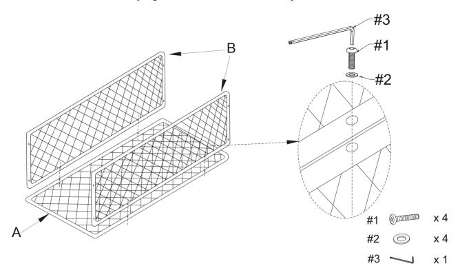
Step 2. Attach end panels (part C) to side panels (part B) using bolts (part #1), flat washers (part #2) and allen wrench (part #3).
