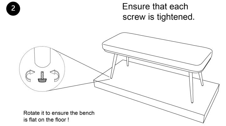
Additional Note About Safety: Bolts may loosen during normal everyday use. They should be periodically inspected and tightened to prevent damage or injury. Always check to be sure that all hardware is kept tightened. Thank you for your purchase.
