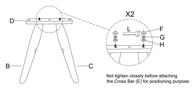
2 Attach the Cross Bar (E) between the Left & Right Leg (B & C).
