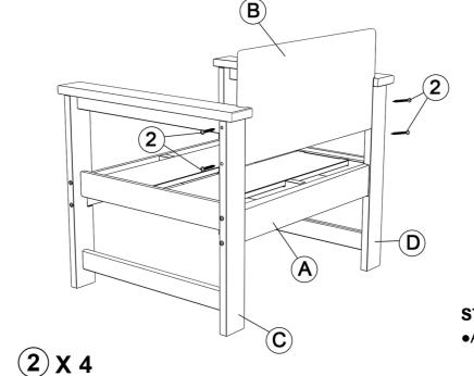
•As shown in the figure, fix D and B,C with 2.
