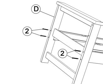
As shown in the figure, Fix A and D with 2
