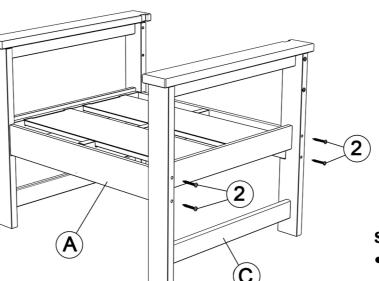
As shown in the figure, Fix A and C with 2
