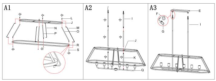
Step A1 » 1) As shown in the figure, the support bar A&B (M&N) and the support tube A&B (O&P) are first fixed to the corresponding position of the top frame (J) with frame nut (L).
