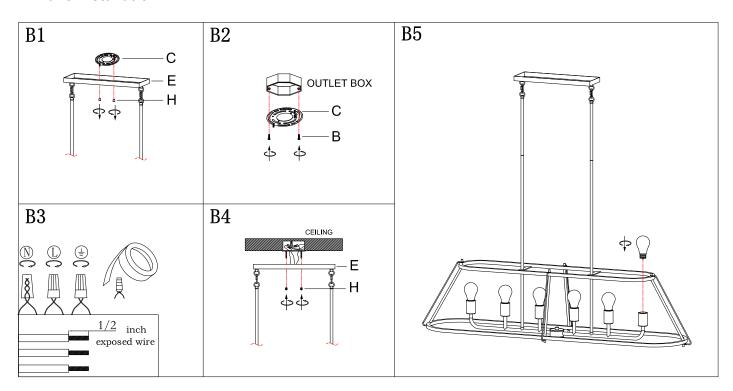
Step B1 » Unscrew ball nuts (H) from mounting plate (C).
